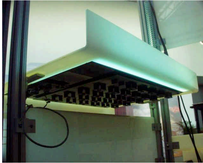
Figure 32. The translucent plastic aids in alignment of sensors under the Origami Desk surface.
